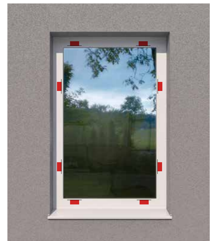
Standard distribution of the I-tec Secure locking points
